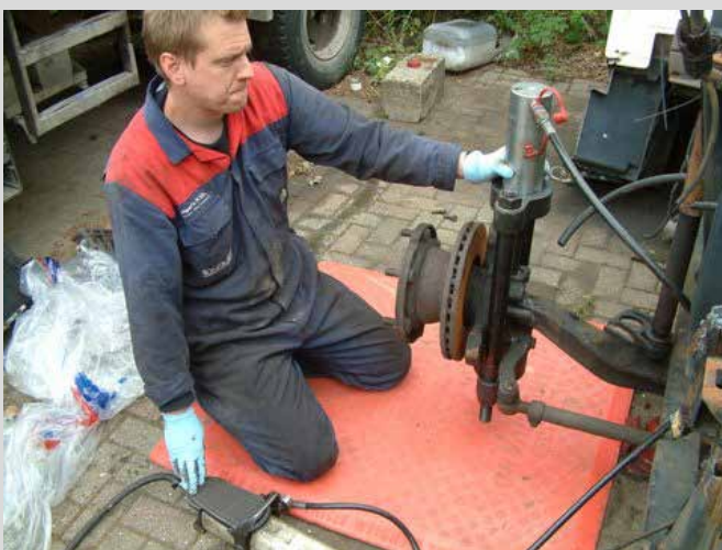
Assemble the KPP20, push the hydraulic pump – the pin pops out. Job done!
